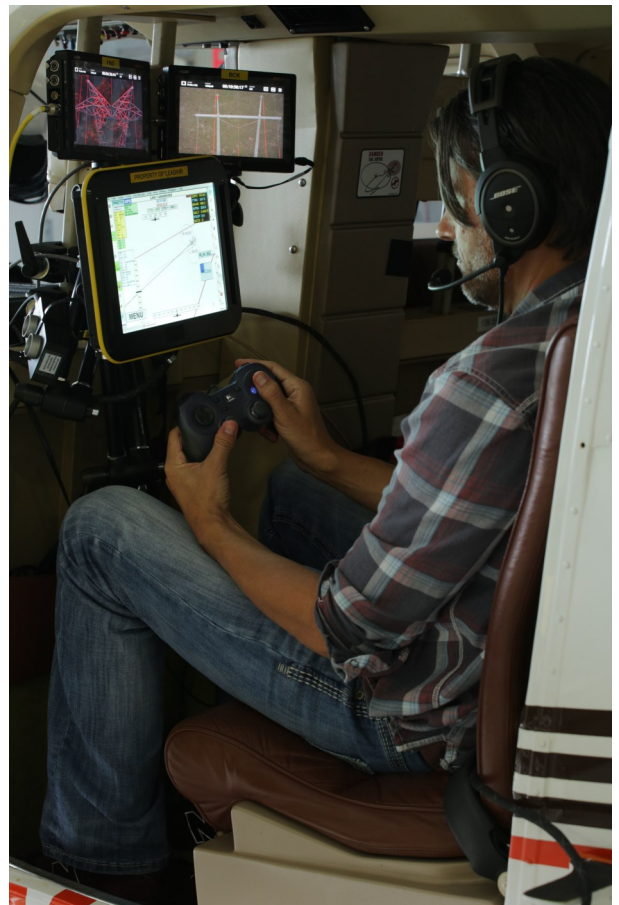
TYPICAL SETUP IN HELICOPTER SHOWING NAVIGATION, VIDEO, AND IMAGE CAPTURE IN REALTIME
